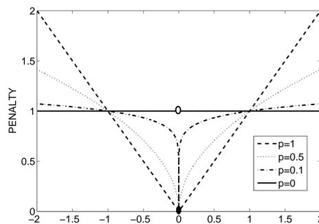
Comparison between cost functions for  $p \leq 1$ . The 0-norm can be seen as more “democratic” than any other norm by weighting all the nonzero coefficients equally.
