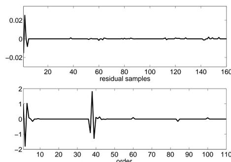
Residual and 110th order linear predictor at the convergence after three iterations. As it is clear, all the information of the speech signal is transferred to the predictor which also show a very clear sparse structure, similar to the convolution between the coefficients of short-term and long-term predictors.
