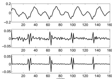
Comparison between true 1-norm 10th order LP residual (middle) and iteratively reweighted 1-norm LP residual (bottom). The original voiced speech is shown on top. Three iterations were performed, sufficient to reach convergence
